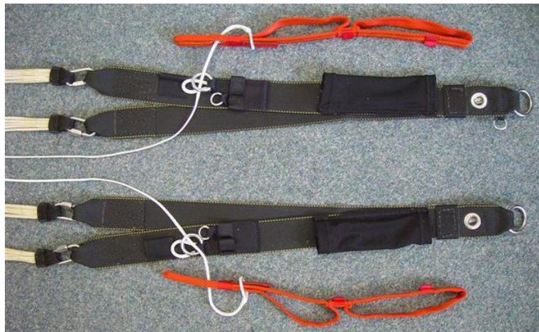
The auxiliary equipment steering loops are placed nearer the centre. The placement and connection is shown in the picture.
