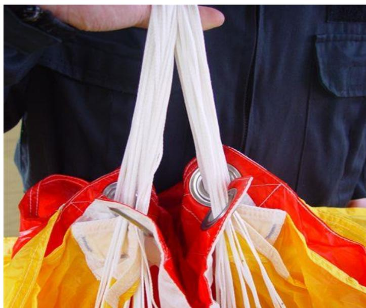
We find the A group of lines on one side of the canopy. We should hold the canopy in front of ourselves, as we have it now, A lines form front part of line groups going through the front passages of the slider (part, which is the closest to us).
