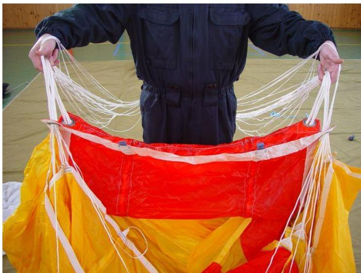
After the lines are checked, connect suspension lines into one joint bundle. Now, place the parachute lines on a random shoulder in such a manner that the stops on the main parachute canopy are at the same height. Use one hand to list individual canopy cells leading parachute edge in an order from A-1 to A-10.
