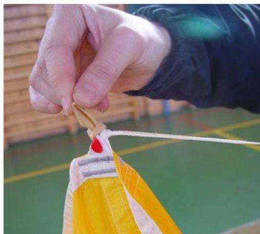
Fold the trailing edge into S-folds in a similar way to stabilizers. Stretch the steering lines and auxiliary steering lines and turn the excess auxiliary steering lines twice around the forefinger and middle finger of left or right hand, and put the resulting twist into a rubber sleeve.
