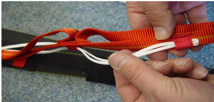
We insert the end of the steering loop to the elastic fabric channel on the riser.
