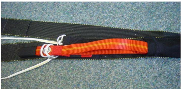
Connection of the auxiliary equipment steering loops of the additional steering RP- 011 TC -1 to the Main riser.
