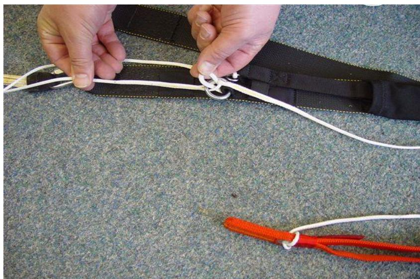
Interlaced brake loop fix by reinforced part of the main canopy steering loops
