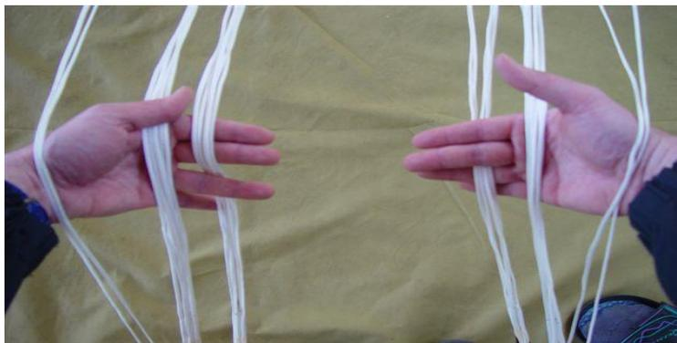
As soon as you reach the canopy edge, stretch out your arms to the sides as much as the slider allows. Shake the canopy several times in order to align single canopy cells. If the canopy is aligned, there will be four clearly differentiated line groups (A, B, C, D) leading up to the stabilizers, where no lines cross one another nor remain twisted. The aim is to get suspension lines aligned with single suspension rib trims.
