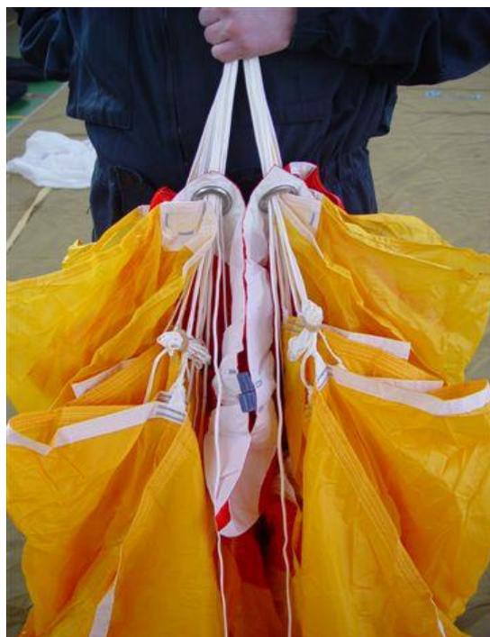
Folds created between individual rows of lines and on the trailing edge should be placed alternately towards the canopy centre, therefore consequent possible shift of some of the suspension lines over the leading canopy side. Folds between suspension lines A and B should on the other hand be folded together with leading canopy edge into its central part. Then we straighten the slider.
