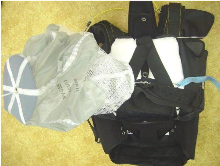
Stow the remaining connection tape as shown in the picture and thread the auxiliary packing cord through the pilot chute.
