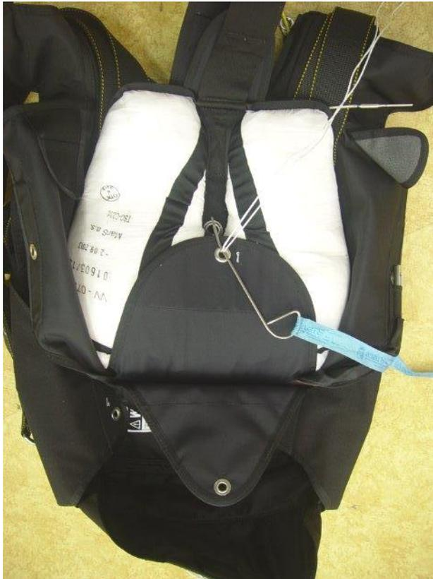
Stow the deployment bag connection tape in the usual way in the shape of the letter “V” under flap no. 1.
