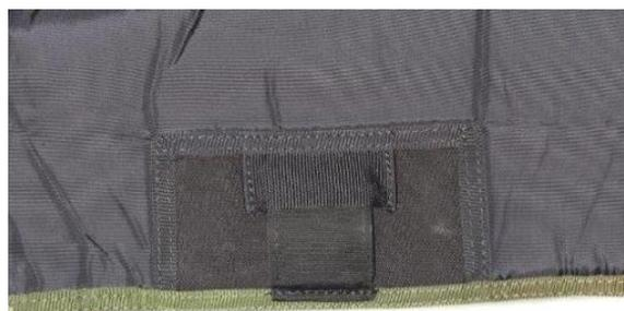
c) Attachment of the pilot chute to the deployment bag webbing
