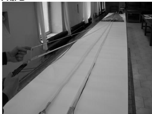
**The suspension lines must not be damaged, worn, or otherwise impaired.**
