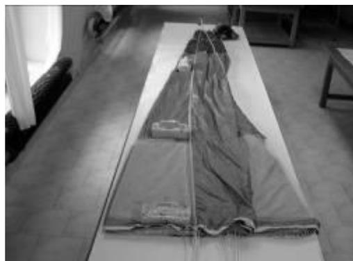
Straighten the canopy along its whole length and inspect the suspension lines. Straighten the lines and inspect them thoroughly from the skirt of the canopy to the SL-01 link connectors. Inspect the lines from all sides
