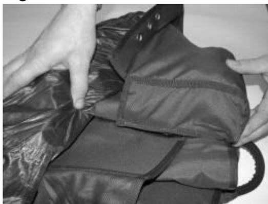
S-fold the bottom (bigger) half of the canopy in the prepared side of the container (Fig. 39 and 39a).
