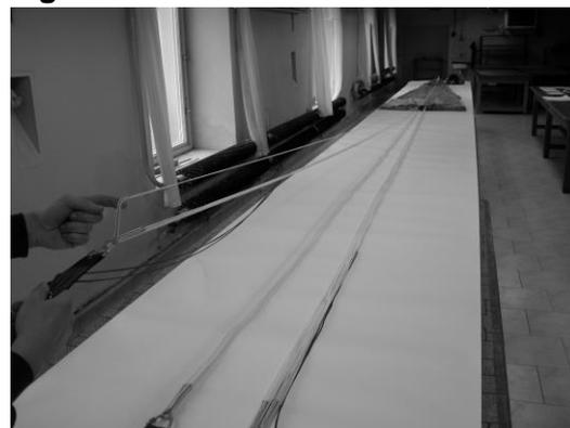
12.1.3 Thread the ripcord cable into its flexible housing. Insert the ripcord handle in the pocket on the harness (Fig. R).
