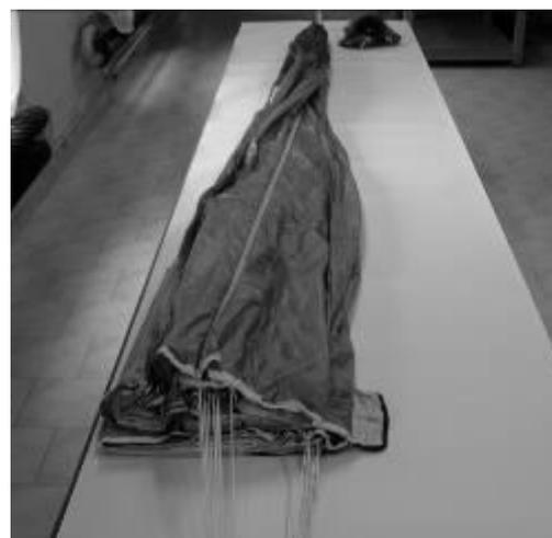
Place line no.12 in the middle of the packing table (Fig.5), place line no.11 on top of line no.12 and continue in the same manner down to line no. 1 (Fig.6, 6a).
