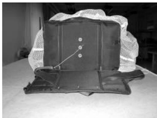
Tuck the pilot chute fabric under the pilot chute (Fig. 72). Turn the rubber rim back down (Fig. 73).
