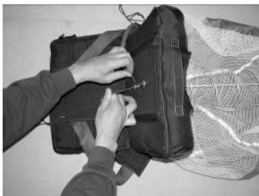
Once the closing cord is secured, cut the temporary tie (Fig. 65).
