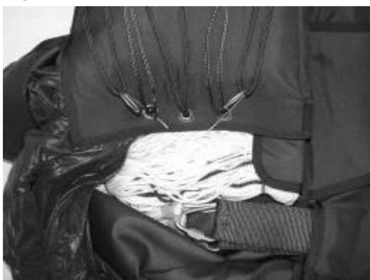
Place the remaining half of the canopy in the opposite side of the container according to the Fig. 43 and 44.
