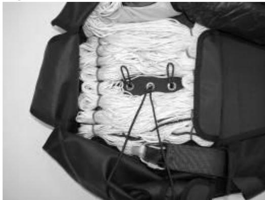
Place pull-up cords in the both temporary locking loops, Fig. 34, 34a.
