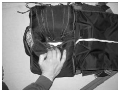
Now, we close the remaining half of the container. Remove one temporary pin and pull the pull-up so that the temporary locking loop appears. Secure the loop with a temporary pin. Repeat the same with the other temporary locking loop.
