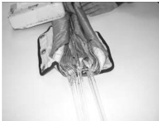
Secure the diaper by stowing the suspension lines (Fig.12, 13, 14, 15, 16).
