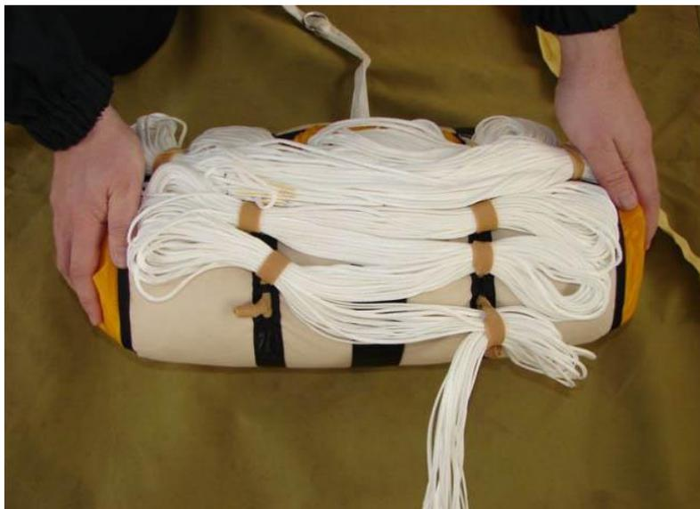
After the suspension lines are put into rubber sleeves on the main canopy deployment bag, smooth the protruding fabric of the canopy into the container together with the remaining suspension lines with harness risers.
