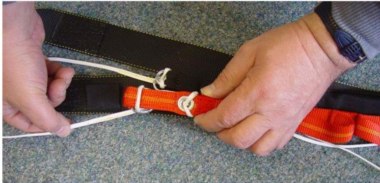
Put the reinforced part of the steering loop into the tape channel on the riser.
