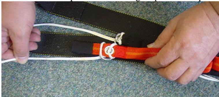
Put the securing reinforcement into the steering loop on the riser.
