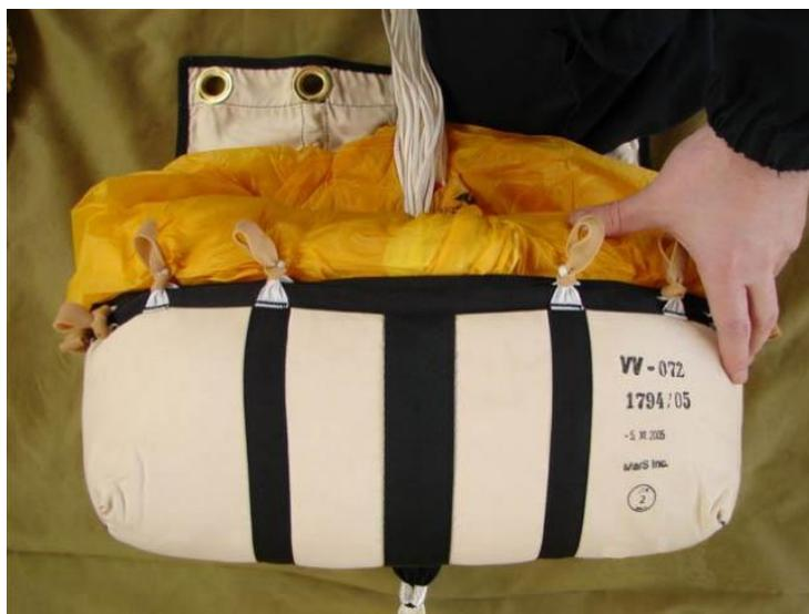
Close the deployment bag with a suspension line bundle. Put the remaining suspension line length into rubber sleeves so that the length of single loop is between 5 and 7 cm.
