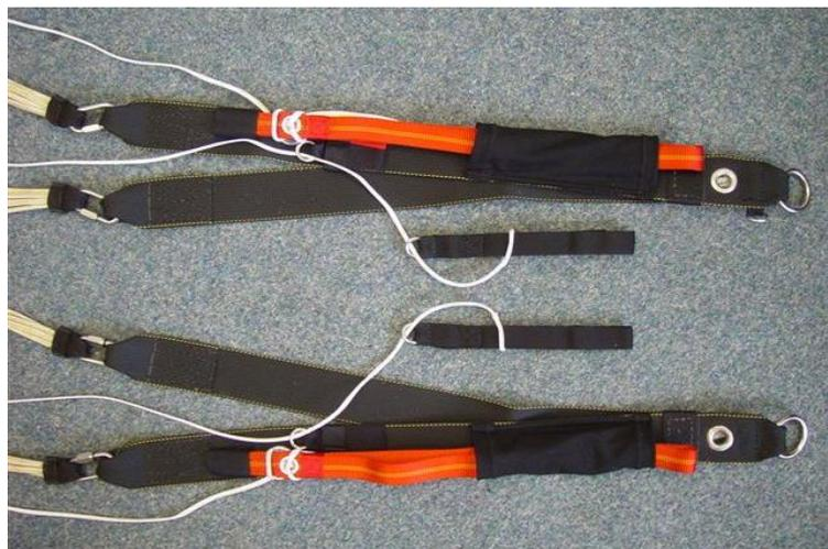
Check a proper connection of the harness risers to the carrying harness and a proper assembly of the three-ring throw-off system.
