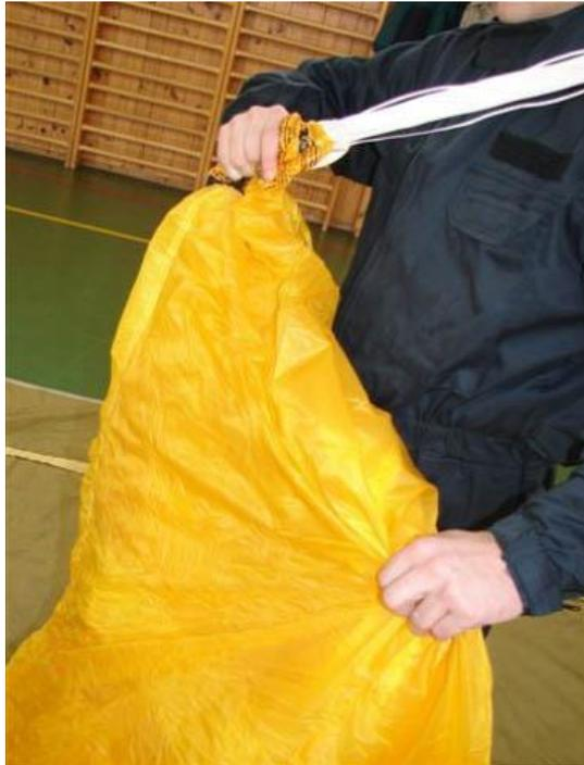
Insert the rolled-up trailing edge part into the parachute centre (see the picture).
