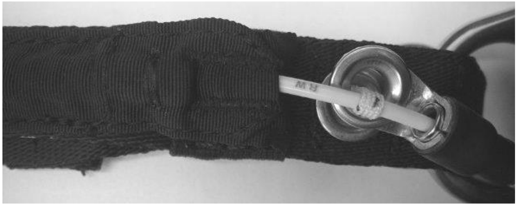
Connected harness riser seen from the bottom
